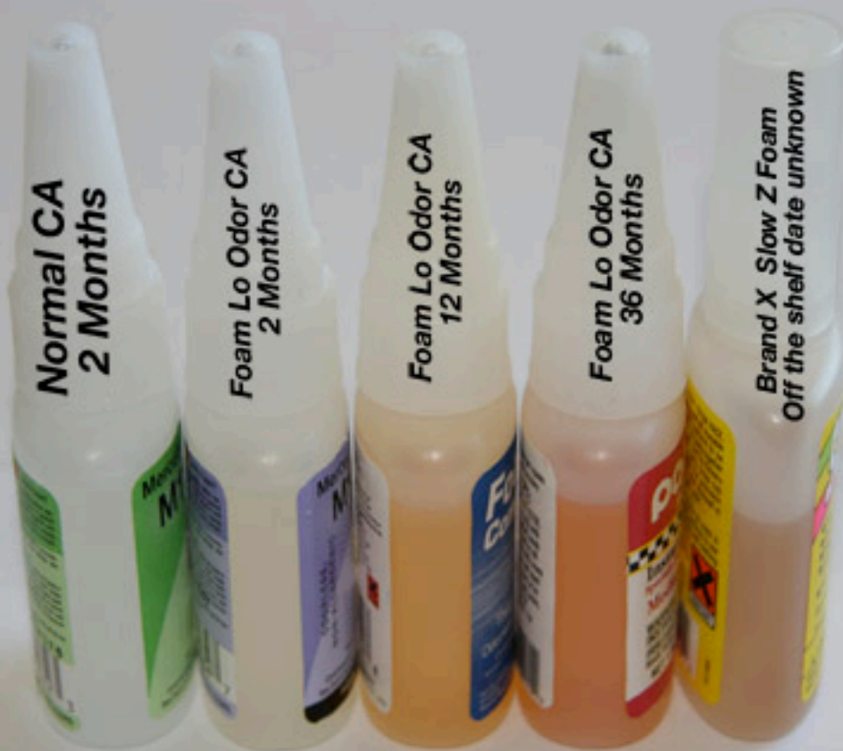
Normal Color changes of Foam Lo Order CA based on time and UV light exposure
